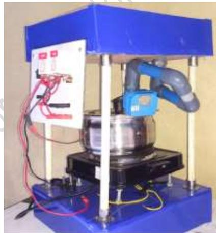
Figure 2. Final prototype of Rasam/Sambar maker
