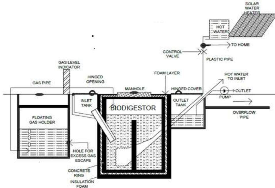
**Figure 1. Improved floating dome biogas digester (named as Udupi Krishna-Manipal or UKM model)**
